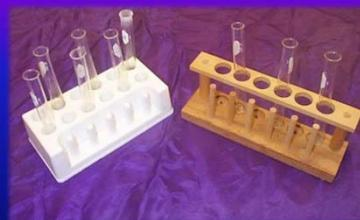
Test tube racks are for holding and organizing test tubes on the laboratory counter. Plastic racks may melt in contact with very hot test tubes.
